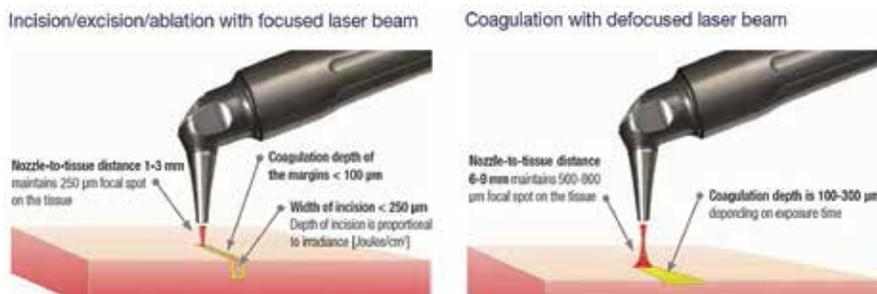
Figure 4: Laser incision/coagulation with focused (250-µm spot size) and defocused (500-800-µm spot size) laser beam delivered from a pen-sized, autoclavable handpiece.
