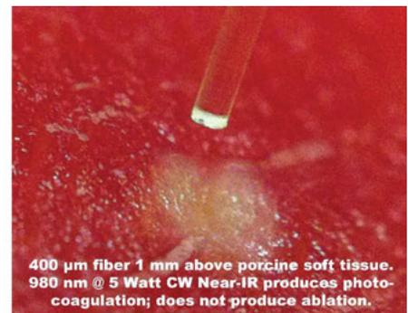
400 μm fiber 1 mm above porcine soft tissue. 980 nm @ 5 Watt CW Near-IR produces photo-coagulation; does not produce ablation.
