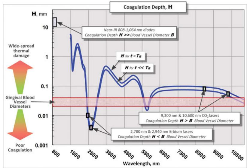
Figure 9: Coagulation depth spectrum for ablation threshold conditions. Logarithmic scale is in use
