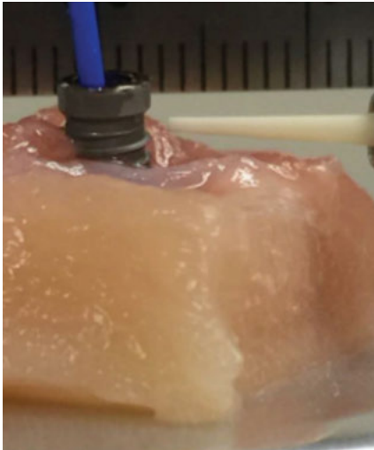
Figure 8: NanoTite™ implant embedded in a block of poultry soft tissue and irradiated by CO 2 laser
